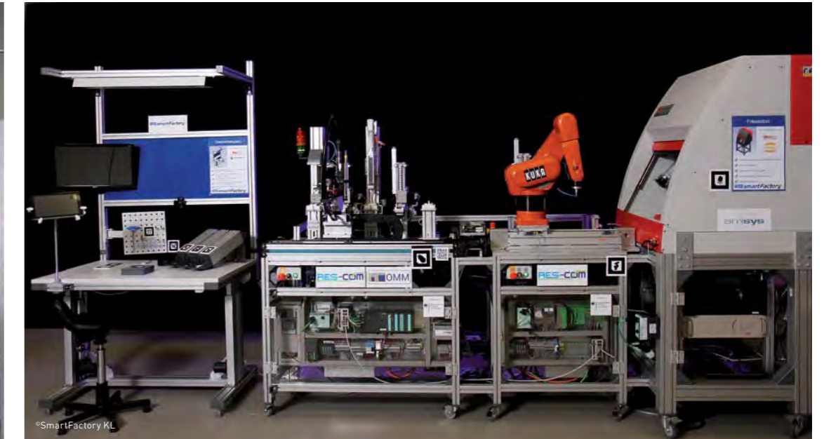
The mobile production plant of the SmartFactoryKL demonstrates the key aspects of INDUSTRIE 4.0: smart product, collaborative machine and augmented operator.
